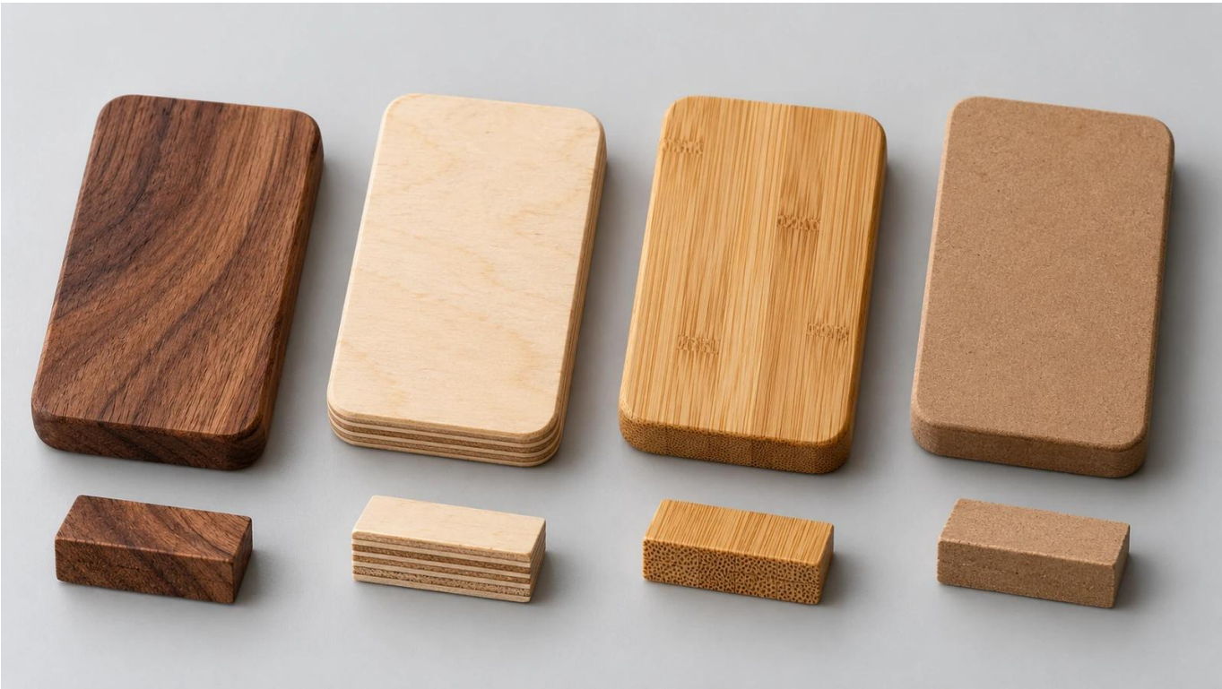
Solid hardwood, plywood, bamboo and MDF behave differently in printing, splitting and moisture exposure.
